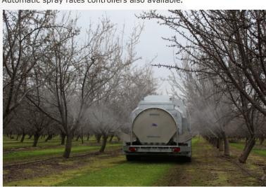
ATOM 4000 comes with diaphragms brass pump for chemicals circuit. Multiple valves system can deliver up to 260 liters/min to the nozzles.
