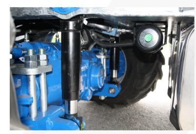
Front + Rear axles hydraulic suspension system. Automatic electronic adjustment of hydraulic suspensions. Automatic leveling of the machine for best stability and comfort.
