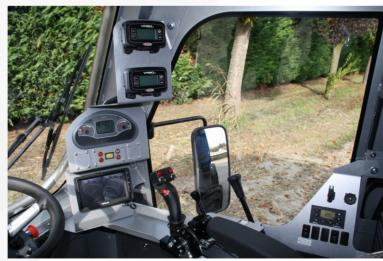
Joystick for forward/reverse and speed control. Switches for nozzles controls directly on main joystick. Electric pressure regulation with switch.
